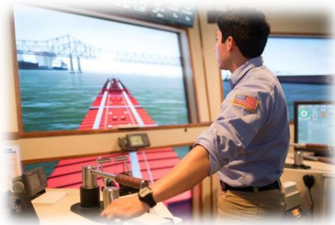
Pictured above is our towboat simulator where wheelhouse crew can gain repetitive practice navigating in extreme conditions and high-risk scenarios
