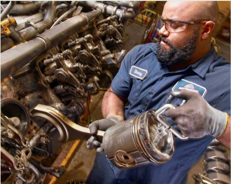
A certified technician at the Stewart & Stevenson Dallas branch removes a piston kit on a MTU 12V4000 during an engine rebuild. Aftermarket services like equipment overhauls and refurbishments, maintenance, and warranty help customers extend the life of their oilfield service equipment.
