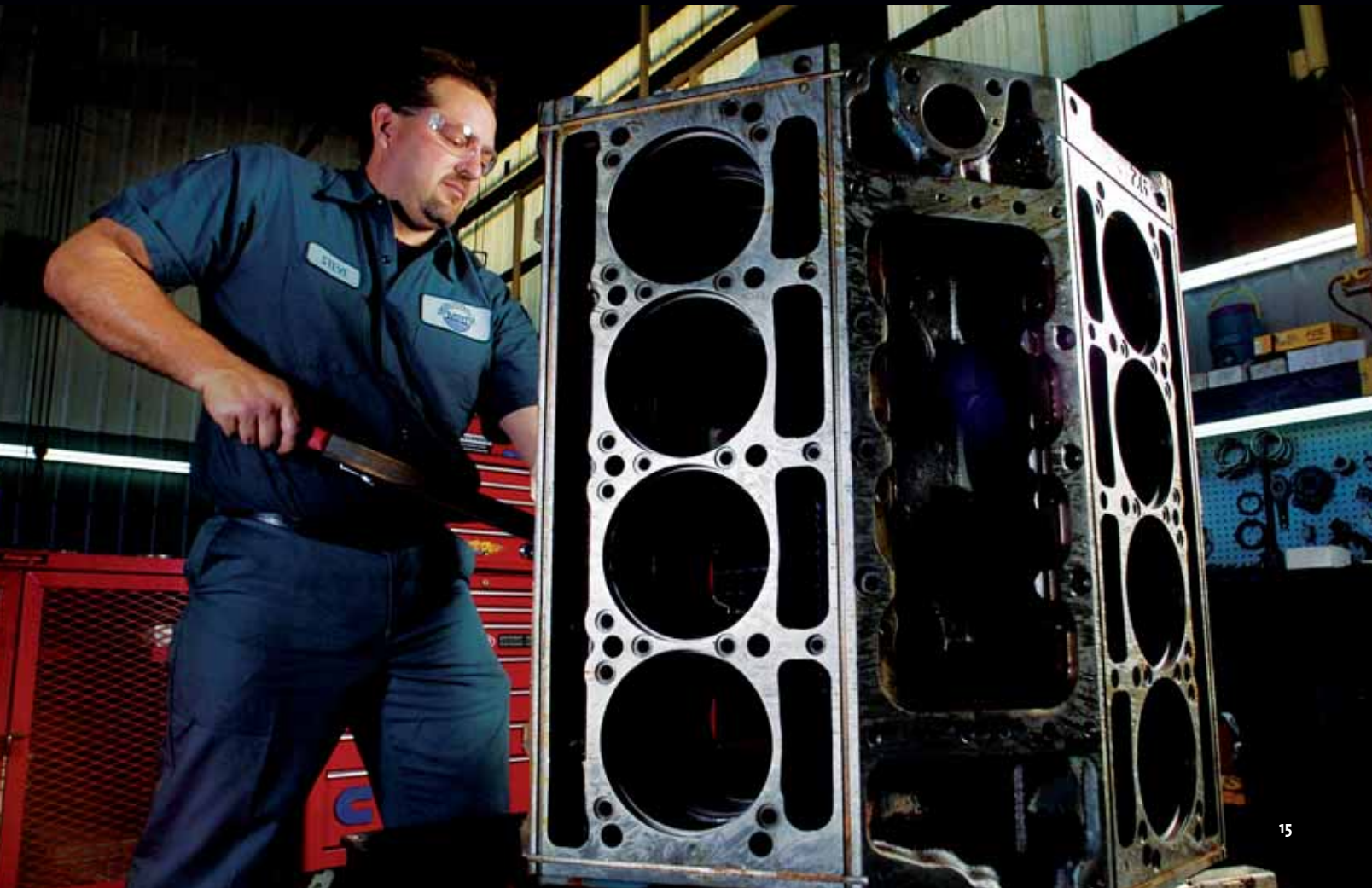
Steve Adams prepares a Detroit Diesel 16V92 rear block as part of the engine rebuilding process. Kirby provides both in-house and in-field service and offers its customers a single source for all their engine, gear and transmission service and parts requirements.
