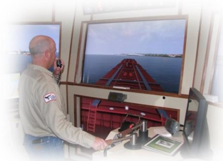
Pictured above is our towboat simulator where wheelhouse crew can gain repetitive practice navigating in extreme conditions and high-risk scenarios
